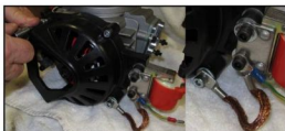
7/ Fit Clutch Cover to Engine using the following three steps. i: Loosely Fit the top two bolts. ii: Fit the lower Clutch Cover Bolt, Earth Cable & Washer. To ensure a good earth the washer must be between the earth cable and clutch cover. iii: Tighten the three Clutch Cover Bolts.
